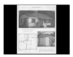
While this "cemestos" house was built with prefabricated cement-and-asbestos panels.
