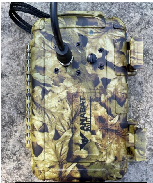
Placement of microphone cable on front cover of Anabat Swift unit.
